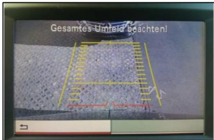
The red guide line indicates the rearmost point of the vehicle to the driver. When reversing, the driver must stop as soon as the red line reaches the obstacle.
