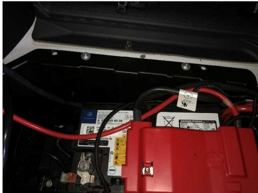
Cable routing through battery box
