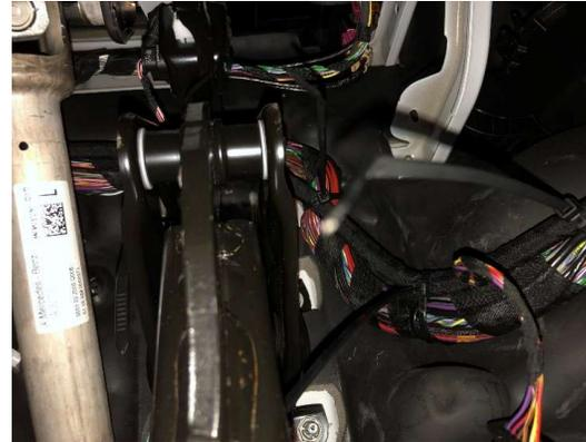
Cable routing over brake pedal assembly
