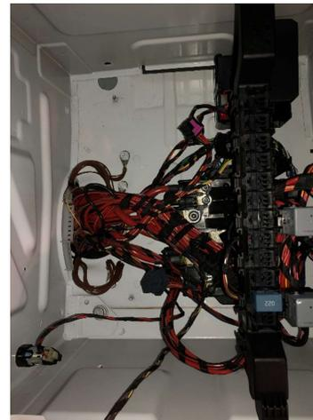
Cable duct into driver's seat base
