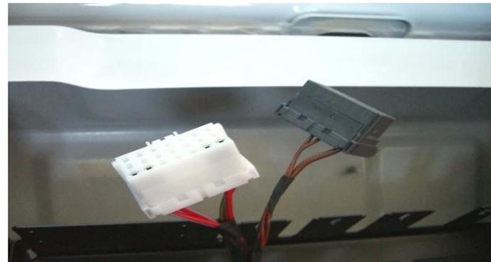
CODE ED8 - PSM pre-wire, located in driver seat pedestal
