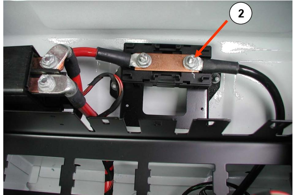
Use position (2) for your electrical connection and install an appropriate fuse as close as possible, ensuring cover (1) is seated properly when closing.
