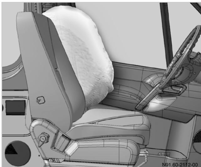
Schematic diagram of deployment area of thorax/pelvis side airbag on left side of vehicle
