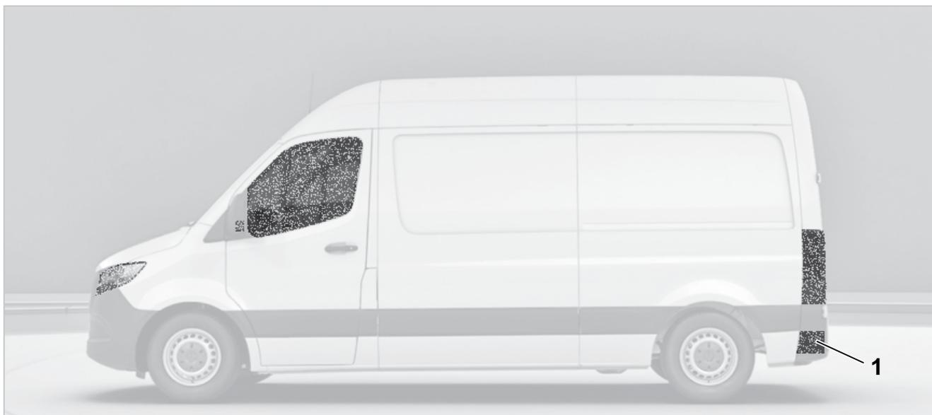
Sides of vehicle - speckled areas: Areas where wrapping is not permissible (example cargo van model designation, schematic diagram)
