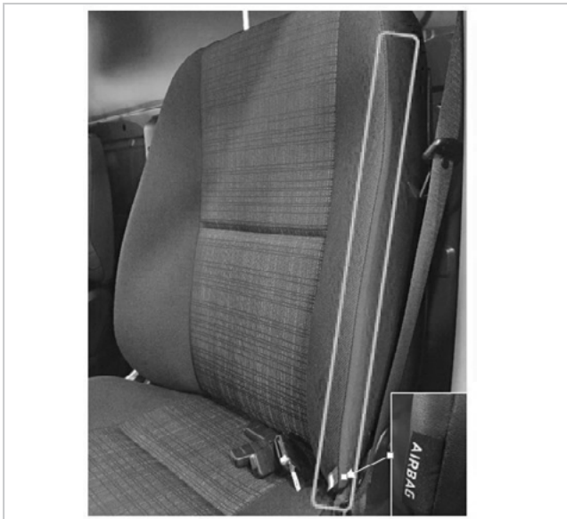
Front Seat with integrated Thorax-Pelvis-Airbag
