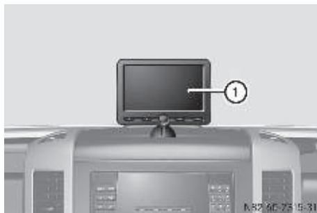
① Rear-view camera monitor
