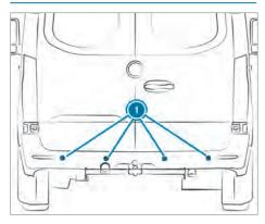
Certain driving and driving safety systems use sensors ① to monitor the area in front of, behind or next to the vehicle (depending on the vehicle's equipment).
