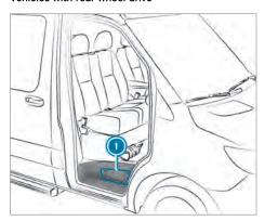
The tire-change tool kit is located in stowage compartment above the step of the co-driver's door and in the stowage compartment in the footwell on the co-driver side.
