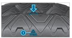
Markings show in which places the bar indicators (arrow) are integrated into the tire tread. They are visible as soon as the tread depth is approximately 1/16 in (1.6 mm).
