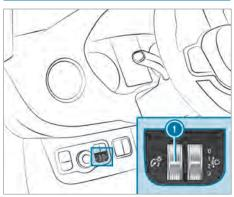
Turn brightness control 1 upwards or down-
