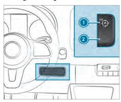
To activate: while the engine is running, press switch 1.
