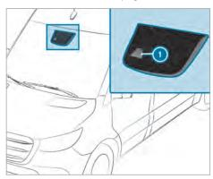
Active Lane Keeping Assist monitors the area in front of your vehicle by means of multifunction camera 1. It serves to protect you against unintentionally leaving your lane. You may also be warned by a noticeable vibration in the steering wheel or by a warning tone and by the status symbol flashing in the Instrument Display. In addition, you may be guided back into your lane by a lane-correcting brake application. A relevant message appears in the Instrument Display.
