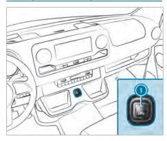
Sliding door button on the center console Sliding door button on the center console
