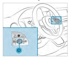
Turn volume control ①. The volume of the current radio or media source is set. The volume of other audio sources can be adjusted separately.
