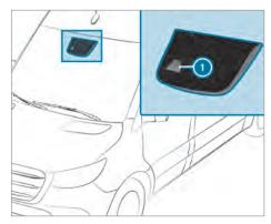
Lane Keeping Assist monitors the area in front of your vehicle with multifunction camera 1. It serves to protect you against unintentionally leaving your lane. You may also be warned by a noticeable vibration in the steering wheel or by a warning tone and by the status symbol flashing in the Instrument Display.
