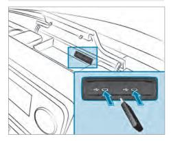
The multimedia connection unit is located at the top center of the storage compartment and has two type C USB ports.
