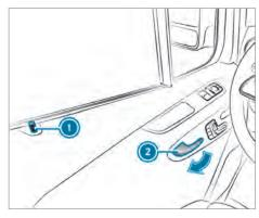
➤ To unlock and open the front door: pull door handle ②.
