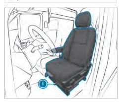
You can rotate the driver's and front passenger seats by 50° and 180°. The seats engage both in and opposite to the direction of travel as well as at 50° towards the exit.
