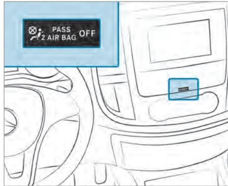
**Self-test of automatic co-driver airbag shutoff**
