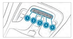
Interior lighting buttons (example: comfort overhead control panel)
