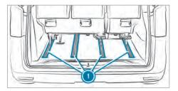
Example: seat rail system with quick-locking mechanism
