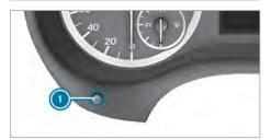
Brightness control (example: vehicle with steering-wheel buttons)
