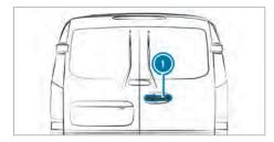
You can stop the rear-end doors at an angle of approximately 90°, and also at 180° or 270°. Make sure that the opened rear-end door is stopped correctly in the catch.
