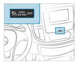
Self-test of automatic co-driver airbag shutoff The PASSENGER AIR BAG OFF indicator lamp lights up for approximately six seconds during the self-test when the ignition is switched on.
