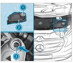
Example: cap and coolant expansion reservoir
