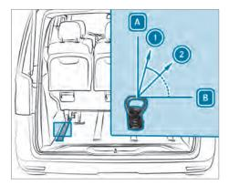
Example: lashing angle for optimal load security
