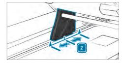
Starting from the basic setting 2, the rear bench seat for passengers can be moved forwards or backwards by 2 in (5 cm). In doing so, make sure that passengers have sufficient legroom to reduce the risk of injury during braking.
