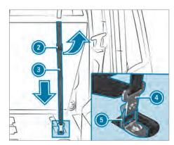
Floor anchorage (example: secured tie-down eye)
