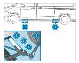
Jacking points (rubber stoppers) are located behind the front wheel arches and in front of the rear wheel arches.
