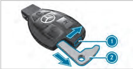
**i** The anti-theft alarm system (ATA) is triggered when you unlock and open the vehicle using the emergency key (→ page 59).
