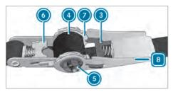
Tensioning lever in the release position
