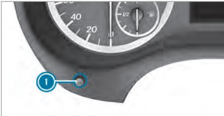
Brightness control (example: vehicle with steering-wheel buttons)
