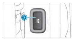
On vehicles with a partition, button (3) is located on the partition next to the doorway at the level of the inside door handle.
