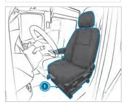
You can rotate the driver's and front passenger seats by 50° and 180°. The seats engage both in and opposite to the direction of travel as well as at 50° to the exit.
