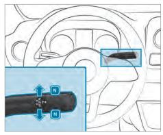
Press the brake pedal and the DIRECT SELECT lever upwards or downwards to the first point of resistance. Transmission position display N is shown in the multifunction display.
