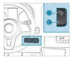
To activate: while the engine is running, press switch 1.
