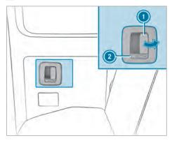
The  $\bigcirc$  symbol indicates that the rear door is unlocked.
