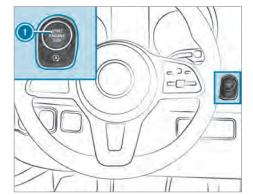
To switch on the power supply: press button (1) once.
