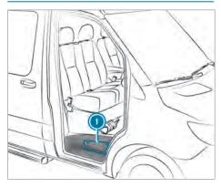
The hydraulic jack is located in side compartment (1) above the co-driver door step.
