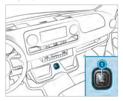
• Opens and closes the sliding door on the right side of the vehicle
