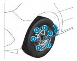
Tighten the wheel bolts or nuts evenly in the sequence indicated (① to ③).
