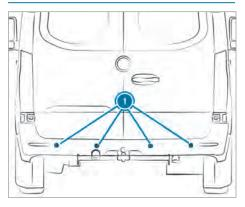
Certain driving and driving safety systems use sensors () to monitor the area in front of, behind or next to the vehicle (depending on the vehicle's equipment).
