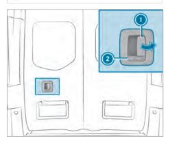
The  $\bigcirc$  symbol indicates that the rear-end door is unlocked.
