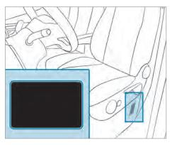
Depending on the vehicle model, the vehicle identification plate is located on the seat base of the driver's seat or on the B-pillar.
