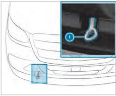
Press the top of the cover and remove the cover.
