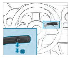
Depress the brake pedal and push the DIRECT SELECT lever downwards past the first point of resistance.
