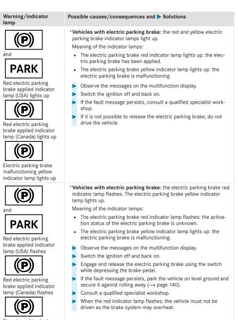
Electric parking brake malfunctioning yellow indicator lamp lights up
