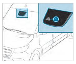
Lane Keeping Assist monitors the area in front of your vehicle with multifunction camera ①. It serves to protect you against unintentionally leaving your lane. You may also be warned by a noticeable vibration in the steering wheel or by a warning tone and by the status symbol flashing in the Instrument Display.
