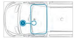
Position of the key holder when the detection range of the antenna is reduced
