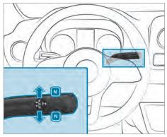
Press the brake pedal and the DIRECT SELECT lever upwards or downwards to the first point of resistance.
