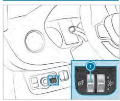
Turn brightness control () upwards or downwards.
