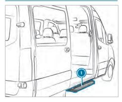
Your vehicle's sliding door may be equipped with an electrical step.
