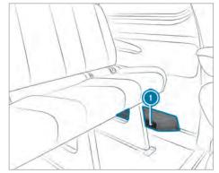
Depending on the vehicle equipment, there will be an air duct or a heater with additional air vents in the rear compartment footwell on the left-hand side (). No objects may be placed there. Occupants must maintain a sufficient distance due to the warm air flow and air intake.
