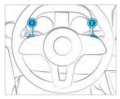
To restrict the shift range: briefly pull steering wheel gearshift paddle ①. The automatic transmission shifts to the next lower gear, depending on the gear currently engaged. The shift range is also restricted.
