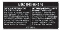
The body builder label is found on the front-end module above the radiator and contains the maximum permissible curb weight for the vehicles.
