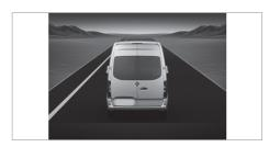
If a front wheel moves onto a detected lane marking, this is highlighted in red on the instrument cluster display in the Assistance menu.
