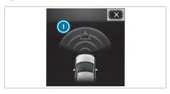
If an autonomous brake application or situationrelated brake force boosting was performed, the pop-up ① appears on the instrument cluster display. It automatically disappears after a short time.
