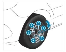
Tighten the wheel bolts or nuts evenly in the sequence indicated (1) to (3).
