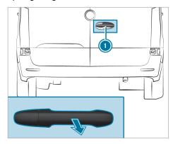
Depending on the respective version of vehicle, the rear-end doors can be locked at an angle of approximately 90° and 270° (side wall).
