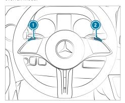
The higher the recuperation, the more sharply the vehicle is braked when coasting and the more electric energy is fed into the high-voltage battery.
