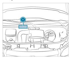
Engraved VIN (1) is located underneath the hood.
