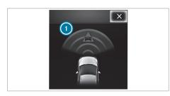
If an autonomous brake application or situationrelated brake force boosting was performed, the pop-up 1 appears on the instrument cluster display. It automatically disappears after a short time.
