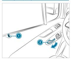
To unlock and open the front door: pull the door handle 2.
