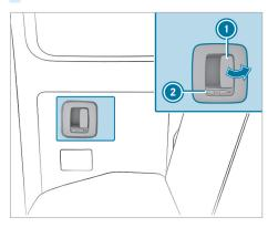
The symbol indicates that the rear door is unlocked.
