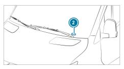
The VIN is also attached as a label on the lower section of the windshield 2.
