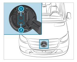
Vehicle socket in the radiator shell
