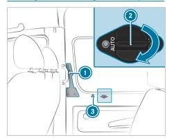
In the event of a malfunction or if the battery has been disconnected, you can use the battery disconnect switch (2) to disconnect the sliding door from the electric motor. You can then open or close the sliding door manually.
