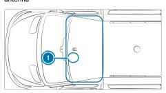
Position of key holder when the antenna detection range is reduced (→ page 103)
