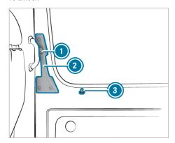
Pull the safety pin ③ upwards manually or use the central locking button to unlock the sliding door (→ page 43).
