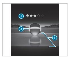
The ECO display shows an evaluation of your driving style on the instrument cluster display depending on the situation. This enables you to check the efficiency of your driving style and adjust it if necessary. The ECO Display menu shows a ball 2 that will roll forwards or backwards in the direction of travel on a stylised road according to the driving characteristics.
