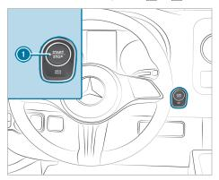
Depress the brake pedal and press button once.
