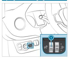
Turn brightness control (1) upwards or downwards.
