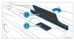
Open the flap of stowage compartment above the media display. With the display facing upwards, place the mobile phone as centrally as possible on the marked surface of mat ②.
