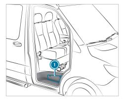
The tire-change tool kit is located in stowage compartment (1) above the step of the front passenger door and in the stowage compartment in the footwell on the front passenger side.
