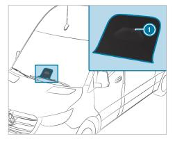
Active Lane Keeping Assist monitors the area ahead of your vehicle with the multifunction camera and can protect you from unintentionally leaving your lane. The system can guide you back into your lane with course-correcting steering interventions, and also warn you with tangible steering wheel feedback.
