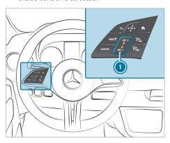
Steering wheel control panel for cruise control
