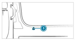
When the sliding door is locked, it can only be opened from the inside by manually unlocking the safety pin (3).
