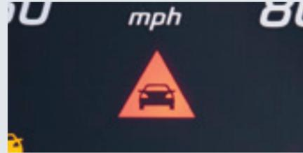
**ACTIVE BRAKE ASSIST<sup>1</sup>** This advanced system senses the likelihood of a collision with a vehicle ahead and sends both a visual and audible warning, and autonomous braking can be initiated.
