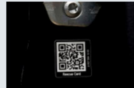
With **RESCUE ASSIST<sup>SM</sup>** first responders to an accident can scan a QR code in a Mercedes-Benz Van to quickly see where batteries, airbags, and other structural elements are located in order to safely perform the rescue.
