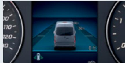
**ACTIVE DISTANCE ASSIST DISTRONIC<sup>5</sup>** This intelligent cruise control system senses traffic conditions and actively controls your speed to keep you at a safe distance.
