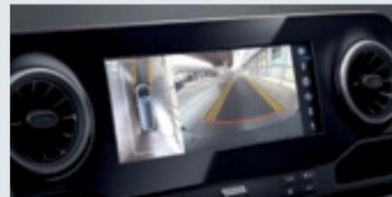
**360° CAMERA<sup>6</sup>** When the Reverse gear is selected, this visual parking aid uses four digital cameras to generate various views of the vehicle's surroundings and show them in real time on the multimedia display.
