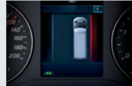
**ACTIVE LANE KEEPING ASSIST<sup>10</sup>** can provide you with visual and audible warnings if your van leaves its lane unintentionally. A camera in the windshield monitors the road ahead and helps detect when you may have veered away from lane markings.
