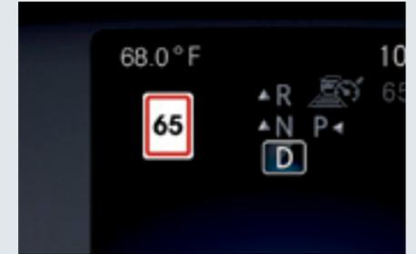
**TRAFFIC SIGN ASSIST<sup>30</sup>** uses a camera to give drivers additional help with identifying speed restriction signs, No Passing zones, and No Entry signs.
