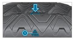
Markings (1) show in which places the bar indicators (arrow) are integrated into the tire tread. They are visible as soon as the tread depth is approximately  $\frac{1}{16}$  in (1.6 mm).
