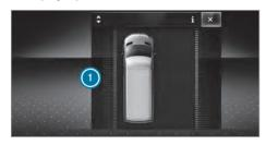
If a lane-correcting brake application from Active Lane Keeping Assist occurs, display (1) appears in the multifunction display.
