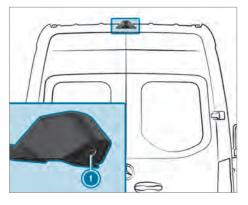
If you have activated the function in the multimedia system, the image from rear view camera 1 appears in the multimedia system when reverse gear is selected. Dynamic guide lines show the path the vehicle will take with the steering wheel in its current position. This helps you to orient yourself and to avoid obstacles when backing up.
