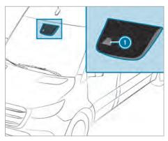
Lane Keeping Assist monitors the area in front of your vehicle with multifunction camera ①. It serves to protect you against unintentionally leaving your lane. You may also be warned by a noticeable vibration in the steering wheel or by a warning tone and by the status symbol flashing in the Instrument Display.
