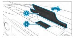
Open the flap of storage compartment ① above the media display. Place the mobile phone as centrally as possible with the display facing upwards on the marked surface of mat ②.
