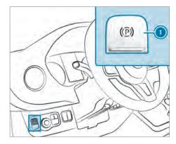
To prevent the electric parking brake from applying automatically, pull switch ①.
