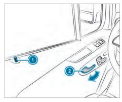
To unlock and open the front door: pull door handle 2.
