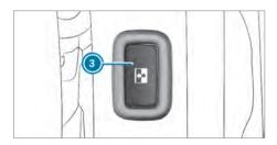
On vehicles with a partition, button **(S)** is located on the partition next to the doorway at the level of the inside door handle.
