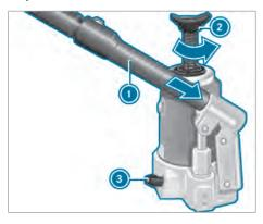
To prepare the hydraulic jack: insert the third rod of pump lever on for the jack into the lug wrench extension.
