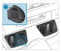
The cup holders for the driver and co-driver are in the center console.
