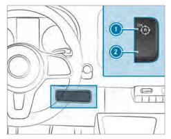
To activate: while the engine is running, press switch (1).
