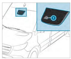
Active Lane Keeping Assist monitors the area in front of your vehicle by means of multifunction camera 1. It serves to protect you against unintentionally leaving your lane. You may also be warned by a noticeable vibration in the steering wheel or by a warning tone and by the status symbol flashing in the Instrument Display. In addition, you may be guided back into your lane by a lanecorrecting brake application. A relevant message appears in the Instrument Display.
