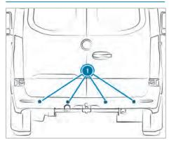
Certain driving and driving safety systems use sensors (1) to monitor the area in front of, behind or next to the vehicle (depending on the vehicle's equipment).
