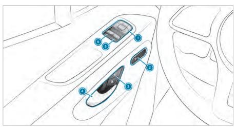
Door control panel of vehicles without electrically adjustable seat
