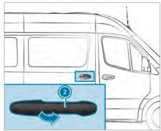
(i) Your vehicle may be equipped with a long sliding door with an intermediate catch. You can also lock the sliding door in place around half-way when opening and closing. If you do this, the door does not have to be opened fully when getting into or out of the vehicle. The sliding door is not fully engaged when in the intermediate catch.
