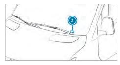
The VIN is also attached as a label on the lower section of windshield 2.
