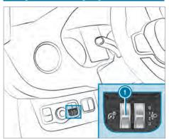
Turn brightness control (1) upwards or downwards.
