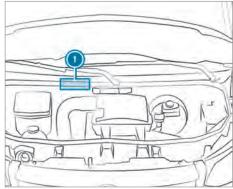
Engraved VIN (1) is located underneath the hood.
