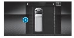
If a lane-correcting brake application from Active Lane Keeping Assist occurs, display 1 appears in the multifunction display.
