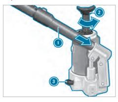
To prepare the hydraulic jack: insert the third rod of pump lever 1 for the jack into the lug wrench extension.
