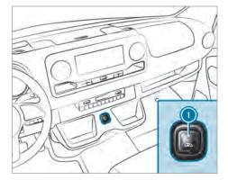
Opens and closes the sliding door on the right side of the vehicle
