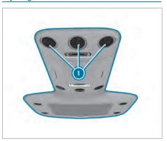
In vehicles with a rear compartment air conditioning system, adjustable air vents have been integrated in the roof air duct.
