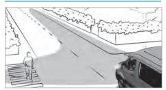
The cornering light improves the illumination of the roadway over a wide angle in the turning direction, e.g. enabling better visibility in tight bends.
