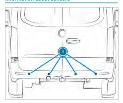
Certain driving and driving safety systems use sensors ① to monitor the area in front of, behind or next to the vehicle (depending on the vehicle's equipment).
