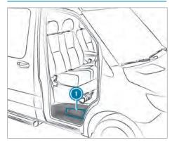
The hydraulic jack is located in side compartment
