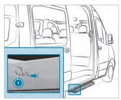
On both sides, insert spring cotters through the housing's holes and into the step as far as they will go.
