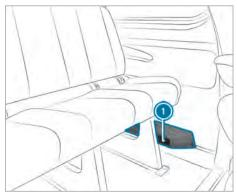
Depending on the vehicle equipment, there will be an air duct or a heater with additional air vents in the rear compartment footwell on the left-hand side ①. No objects may be placed there. Occupants must maintain a sufficient distance due to the warm air flow and air intake.
