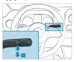
The automatic transmission shifts through the individual gears automatically when it is in transmission position  $\boxed{\textbf{D}}$ . This is determined by the following factors:
