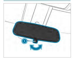
Fold anti-glare lever (1) in the direction of the arrow.
