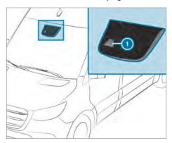
Active Lane Keeping Assist monitors the area in front of your vehicle by means of multifunction camera ①. It serves to protect you against unintentionally leaving your lane. You may also be warned by a vibrating message from the steering wheel and by the status symbol flashing in the instrument display. In addition, you may be guided back into your lane by a lane-correcting brake application. A relevant message appears in the instrument display.
