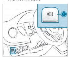
To prevent the electric parking brake from applying automatically, pull switch .
