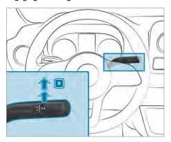
Depress the brake pedal and push the DIRECT SELECT lever upwards past the first point of resistance. Transmission position display R is shown in the multifunction display.
