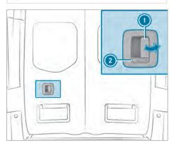
The graph symbol indicates that the rear-end door is unlocked.
