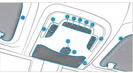
Overhead control panel for vehicles with bus equipment  $\bigcirc$  Switches the rear interior  $\rightarrow$ Sun visors lighting on/off ② ✓ Breakdown assistance call button ③ 盗 Switches the right-hand reading light on/off Activates/deactivates 86 the bus function Switches reading lights in the passenger compartment on/off reading light on/off (ii) Glasses compartment 86 (5) Switches automatic light control on/off Switches the front interior lighting on/off
