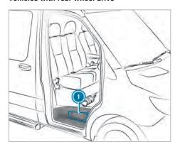
The tire-change tool kit is located in stowage compartment 1 above the step of the co-driver's door and in the stowage compartment in the footwell on the co-driver side.
