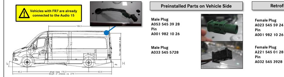
After the camera has been connected, it is merely necessary to add Code FR8 using the Star diagnostic system so the radio recognizes that a camera is connected. The radio receives the signal from the transmission via the CAN bus. If the static guiding lines on the monitor do not correspond to the rearmost point of the vehicle (this will not generally be the case as these are adapted to the factory camera FR8), the lines can also be deleted with Code O43 using the Star diagnostic tool.
