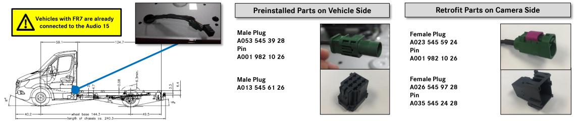
After the camera has been connected, it is merely necessary to add Code FR8 using the Star diagnostic system so the radio recognizes that a camera is connected. The radio receives the signal from the transmission via the CAN bus. If the static guiding lines on the monitor do not correspond to the rearmost point of the vehicle (this will not generally be the case as these are adapted to the factory camera FR8), the lines can also be deleted with Code O43 using the Star diagnostic tool.
