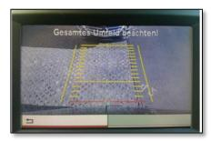
The red guide line indicates the rearmost point of the vehicle to the driver. When reversing, the driver must stop as soon as the red line reaches the obstacle.
