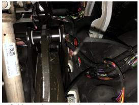
Cable routing over brake pedal assembly
