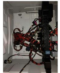
Cable duct into driver's seat base
