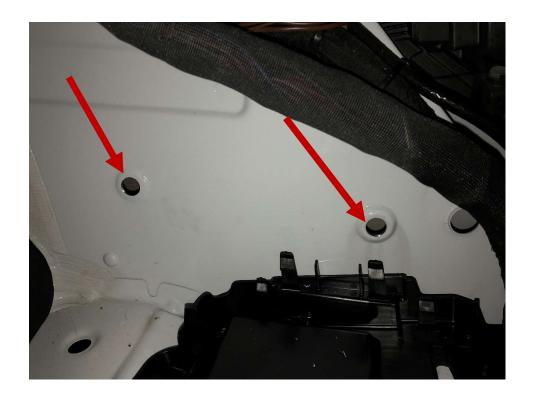
1. Install battery bracket (A9075402505) as shown below using nut (N000000003477) and bolts
