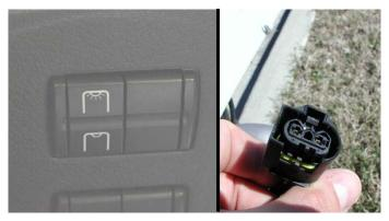
CODE L72 - Instrument panel switch and wiring on rear crossmember. The interface supports bulb loads up to a maximum of 4 amps and ohmic loads up to a maximum of 10 amps.
