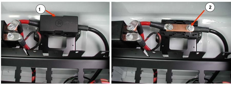
If an aux battery (code E28) is installed an electrical connection is located inside the driver seat pedestal. Please remove cover (1).
