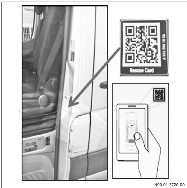
Attachment (example) of QR code rescue sticker on left B-pillar (schematic diagram)
