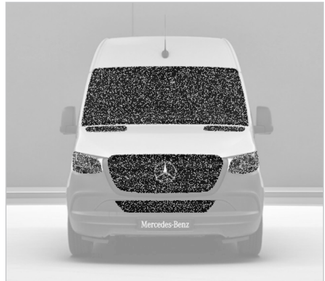
Front of vehicle - speckled areas: Areas where wrapping is not permissible (example cargo van model designation, schematic diagram)
