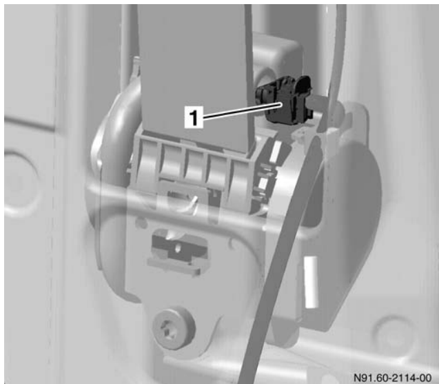
Retractor with pyrotechnic belt tensioner
