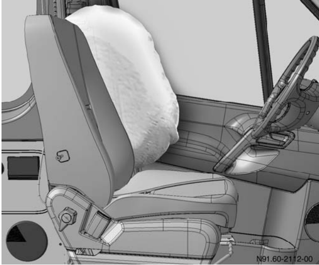
Deployment area of left-hand side thorax bag
