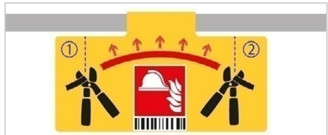
High-voltage rescue disconnect device information label (extract from rescue card)
